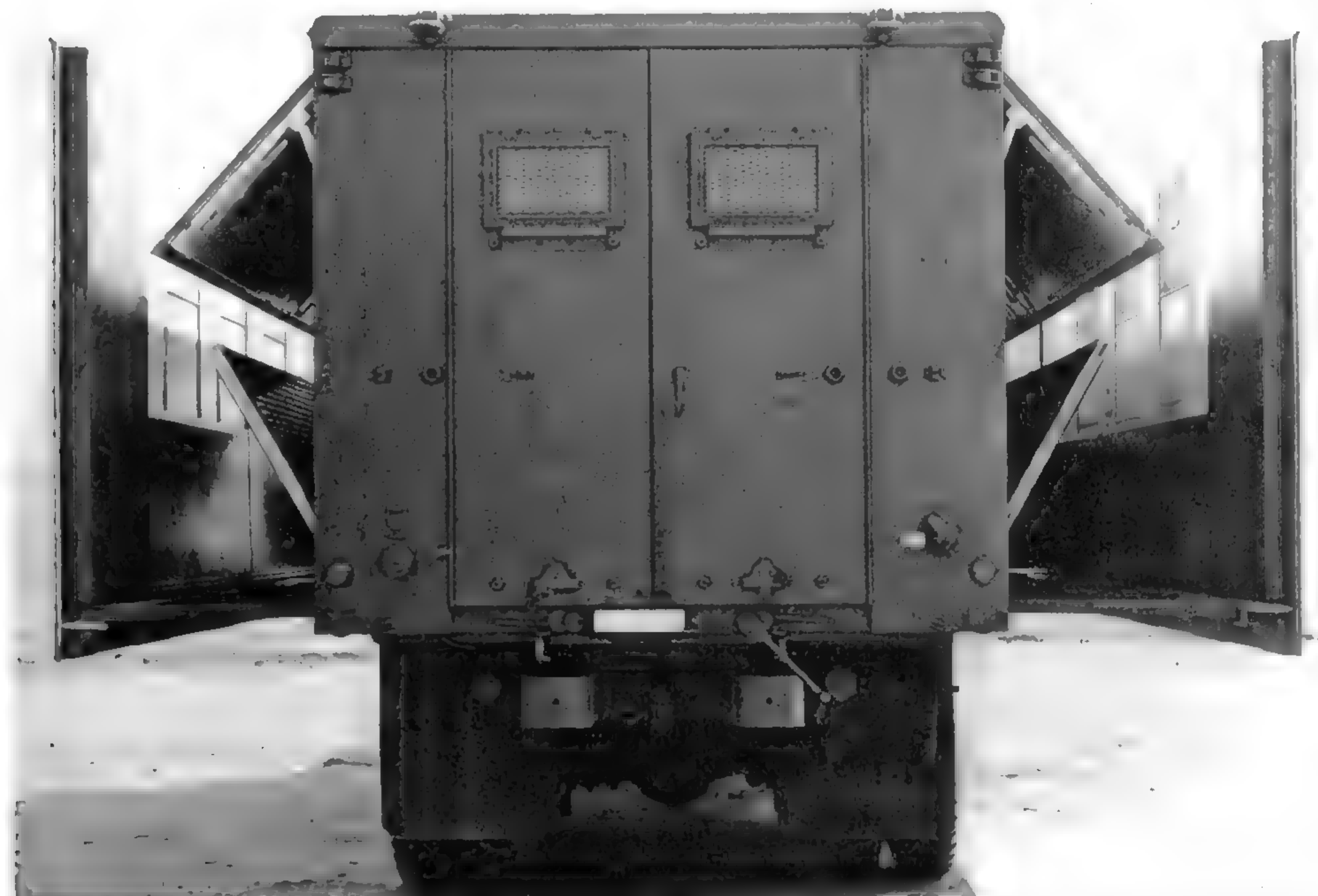
This photo, taken during the XM292 expansion process, shows the sides partially cranked out, and the roof and floor sections swinging into place. (National Archives and Records Administration photo)
